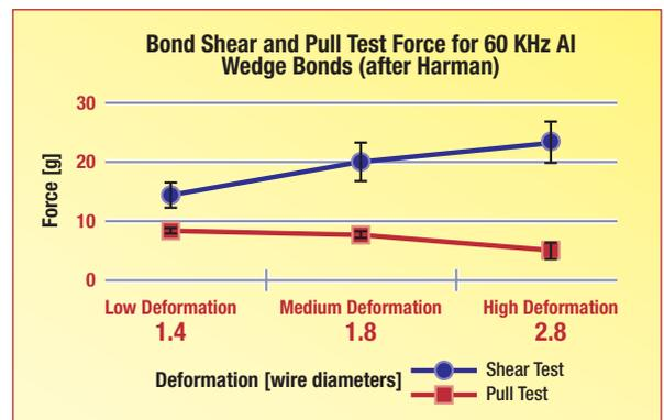
This graphic demonstrates why shear testing and pull testing must both be employed. (After G. Harman, *Wirebonding in Microelectronics*, McGraw-Hill, 1997, p. 105.)
